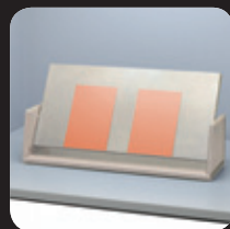
Sample holder with 5 angled adjustments (-15°, 0°, 15°, 45°, 60°)
