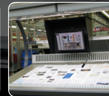
The "Scroll" solution: movable monitor with position sensor for displaying zone by zone areas of the press sheet.
