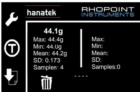
The bin icon is shown allowing the user to discard the last test result. Pressing and holding the button will delete all the samples.
