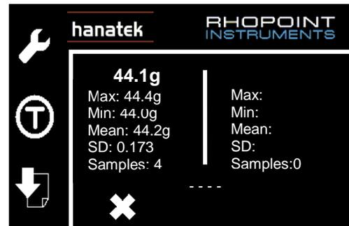
When the countdown timer has finished the X will show at the bottom of the screen indicating the jaw needs to be returned.
