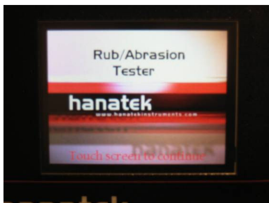
The touch screen display after switch on. Press anywhere on the screen to continue.
